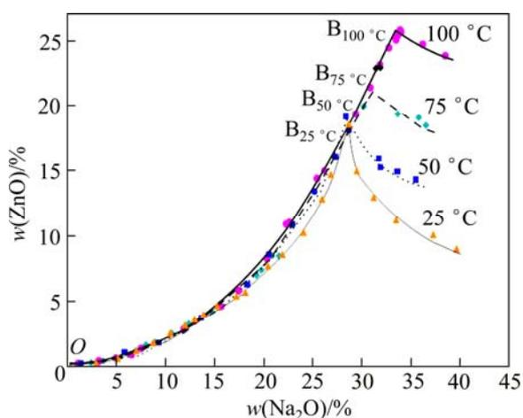
Fig. 3 Solubility of zinc in  $\text{Na}_2\text{O}-\text{ZnO}-\text{H}_2\text{O}$  system
