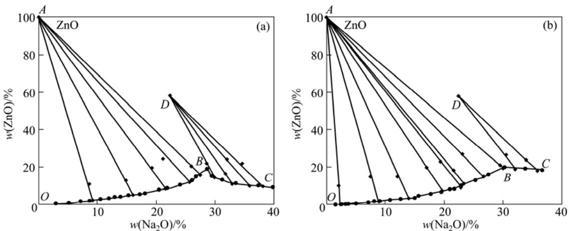
Fig. 1 Equilibrium diagram of  $\text{Na}_2\text{O}$ –ZnO– $\text{H}_2\text{O}$  system at 25 °C (a) and 75 °C (b)
