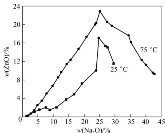
Fig. 4 Solubility of zinc oxide in  $\text{Na}_2\text{O}-\text{ZnO}-\text{H}_2\text{O}$  system by URAZOV et al
