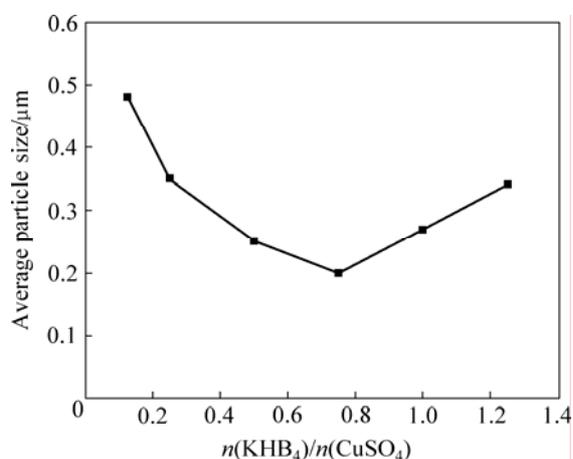
**Fig.1** Effect of molar ratio of  $\text{KBH}_4$  to  $\text{CuSO}_4$  on average particles size
