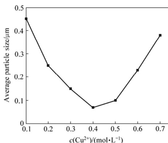
**Fig.3** Effect of concentration of copper ions on average particle size of copper
