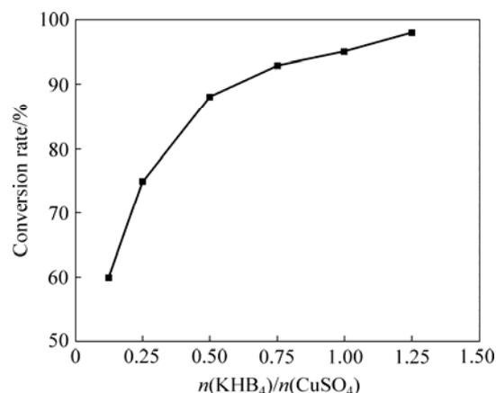
**Fig.2** Effect of molar ratio of  $\text{KBH}_4$  to  $\text{CuSO}_4$  on conversion rate
