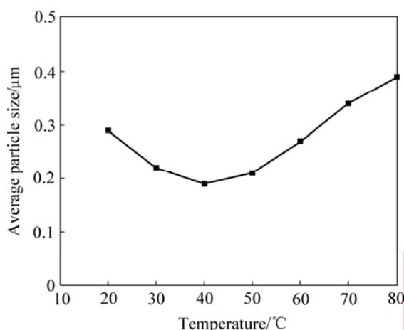
**Fig.4** Effect of reaction temperature on average particle size of copper
