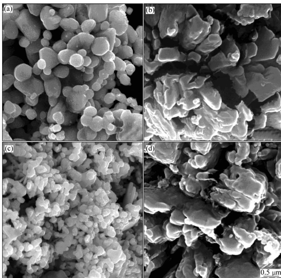
**Fig.5** SEM images of copper powders prepared with different dispersing agents: (a) Polyvinyl pyrrolidone; (b) Glycerol propanetriol; (c) *n*-butyl alcohol; (d) PEG-400
